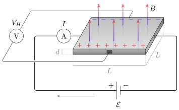
A longitudinal emf  $\mathcal{E}$  is applied to the plate. At steady state, a Hall voltage  $V_H$  is measured across the plate due to the buildup of charge on either side of the plate. If the electrical resistivity of the plate at zero magnetic field is  $\rho_0$ , what is the Hall voltage  $V_H$  and the current I through the plate? Express your answer in terms of  $\rho_0$ ,  $\mathcal{E}$ , B, and the dimensions of the plate.
