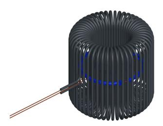
The ABRACADABRA<sup>1</sup> experiment, currently taking data at MIT, is a toroidal solenoid with inner and outer radius  $R_{\rm in}$  and  $R_{\rm out}$  and height h. You may assume  $h \gg R_{\rm out}$  for simplicity. A superconducting wire carrying current I wraps N times around the toroid, where N is high enough to neglect the discreteness of the wires. A circular pickup loop with radius slightly less than  $R_{\rm in}$  is placed at the center of the toroid.
