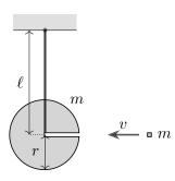
A uniform ball of mass m and radius r is attached to a massless rigid rod, so that its center is a distance  $\ell$ from the ceiling. The ball has a small tunnel hollowed out. A small block of mass m and speed v goes into the tunnel and collides at the center of the ball, perfectly inelastically. Subsequently, to what maximum height does the block rise?
