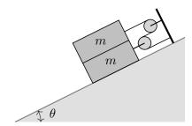
Suppose that the coefficient of static friction between the lower block and the slope is  $\mu$ , and all other surfaces are frictionless. What is the minimum value of  $\mu$  so that the blocks can stay static?
