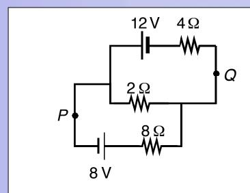
Calculate current in  $2-\Omega$  resistor and potential difference between P and Q.
