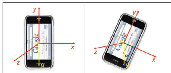
Fig. 3. The orientation of the three independent acceleration sensors of an iPhone or iPod touch; the sensors measure the acceleration in the direction of the three plotted axes.
