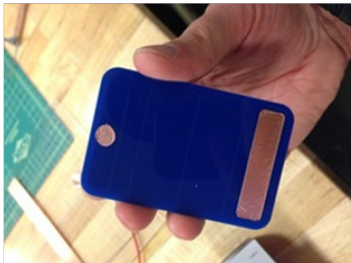
A simple capacitor made in the Fabrication Laboratory
