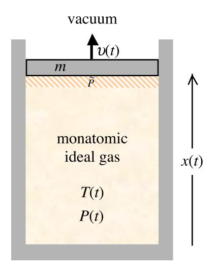
The bulk of the gas has time-varying pressure P, absolute temperature T, and volume V = Ax. However, the gas atoms next to the piston (occupying the hatched slice of negligible volume compared to V) exert dynamic pressure  $\tilde{P}$  on the piston.
