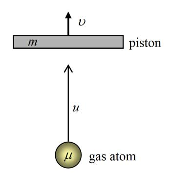
A gas atom of mass  $\mu$  and upward velocity u makes an elastic collision with the piston of mass m and upward velocity v, where  $m \gg \mu$  and  $u \gg v$ .
