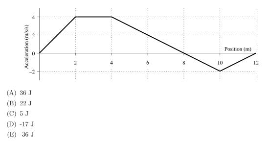
11. A 2.25kg mass undergoes an acceleration as shown below. How much work is done on the mass?
