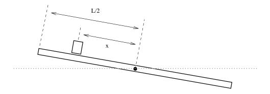
Let x be the displacement of the block along the plank, as measured from the pivot, and let  $\theta$  be the angle between the plank and the horizontal. You may assume that centripetal acceleration of the block is negligible compared with the linear acceleration of the block up and down the plank.
