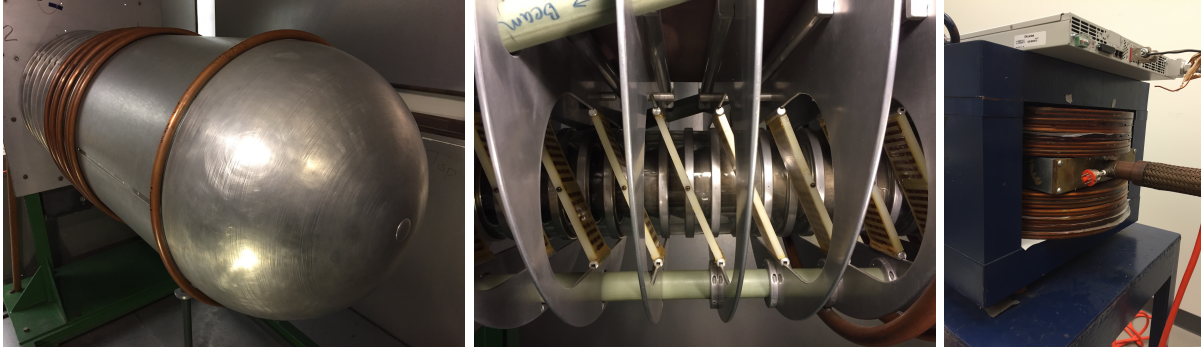
Accelerator dome (assume it is a sphere); accelerating column; bending electromagnet
