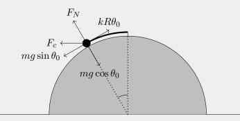
Here,  $F_c = \frac{mv^2}{R\sin\theta_0}$  is the centrifugal force, and  $F_r$  is the radial force from the hemisphere. The forces in the radial direction must balance for the mass to be constrained to the surface of the sphere. Thus,
