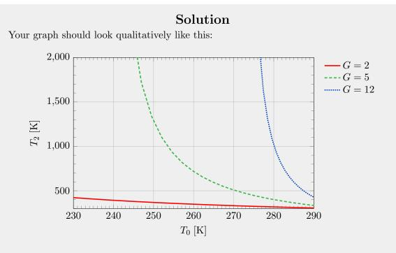
The intuition for the curves is that the efficiency gain becomes high when  $T_1$  gets close to  $T_0$ , and it becomes low when  $T_2$  gets close to  $T_0$ .
