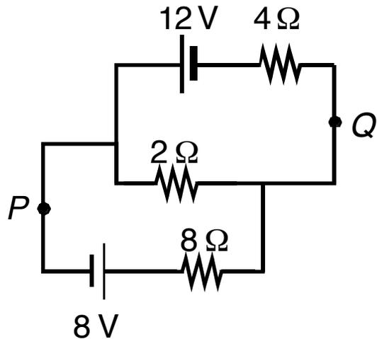
Calculate current in 2- $\Omega$  resistor
