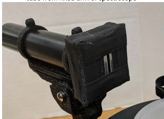
Tape and inserted onto inner tube of spectroscope
