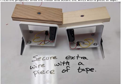
10. Install the batteries. Reverse the battery polarity to reverse the fan direction. Secure batteries with tape if needed.
