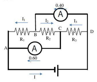
By junction rule at B:  $I_1 + I_2 = 0.40A$ By junction rule at C:  $I_2 + I_3 = 0.60A$
