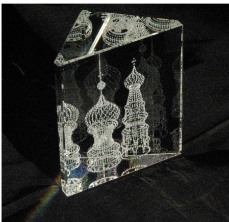
Fig. 2. Three-dimensional image within a glass prism purchased by the author in Russia in 1995. Each microscopic glass bubble was created by a single pulse from a laser beam focused to a point. The nonlinear optical process of multiphoton ionization results in localized plasma formation and internal melting. This image was created on a lathe; today with computer control any 3D image can be inscribed inside a block, with a process that originates from nonlinear optics. See Ref. 143.
