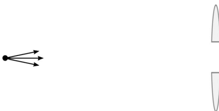
Fig. 4. Split image. A point source of monochromatic light placed at a distance greater than the focal length of a converging lens produces an image point on the far side of the lens. When the lens is split into two halves as shown, two image points are produced. These coherent image points can create interference fringes on a distant screen.
