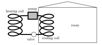
Assume that the outside air temperature is  $T_H$  and the inside air temperature is  $T_L$ . The air-conditioner unit consumes electric power P. Assume that the air is sufficiently dry so that no condensation of water occurs in the cooling coils of the air conditioner. Water boils at 373 K and freezes at 273 K at normal atmospheric pressure.
