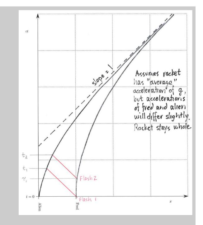
If you had assumed (somewhat incorrectly) that the two ends of the ship have the same acceleration, then the two trajectories would be approaching two different asymptotes separated by a constant horizontal distance. But this would mean the apparent length of the ship was constant, regardless of speed. In the instantaneous rest frame of the ship we then require that Fred and the Alien be moving apart. This means that the ship must be stretching, and eventually breaking.
