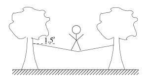
The Young's modulus is defined as the ratio of stress to strain, where stress is the force applied per unit area and strain is the fractional change in length  $\Delta L/L$ . The cable's Young's modulus is
