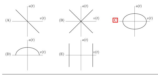
By conservation of energy,  $E = kx^2/2 + mv^2/2$ . In addition, the acceleration is a = -kx/m, which implies that  $E = k(ma/k)^2/2 + mv^2/2$ . Therefore, when a is plotted against v, the result is an ellipse. All combinations of signs of a and v are possible, so the ellipse occupies all four quadrants, giving choice (B).
