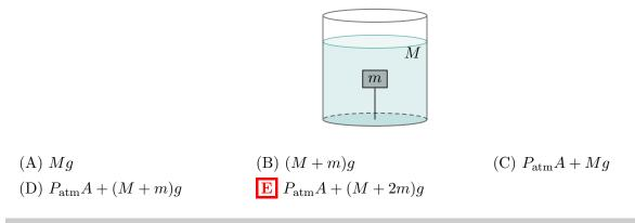
Consider force balance on the system of the block and water. The atmospheric pressure applies a downward force  $P_{\text{atm}}A$ , and gravity applies a downward force (M + m)g. Now, the buoyant force on the block is 2mg because water is twice as dense, which means the string applies a downward tension force mg to keep the block in place. To balance all these forces, the base of the cup must exert an upward force  $P_{\text{atm}}A + (M + 2m)g$ .
